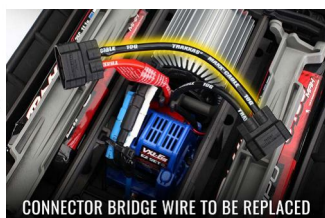
Connection Bridge Wire To Be Replaced
